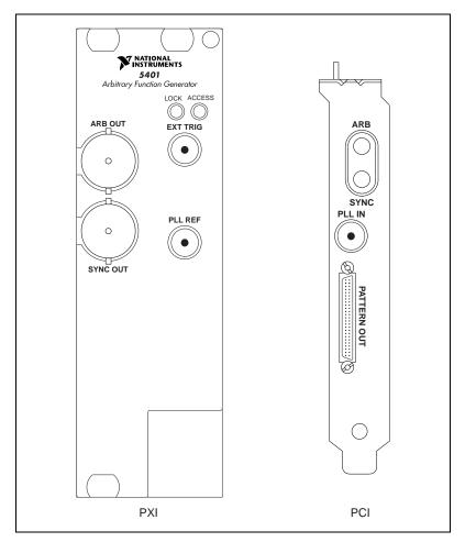
Figure 1-1. NI 5401 I/O Connectors
